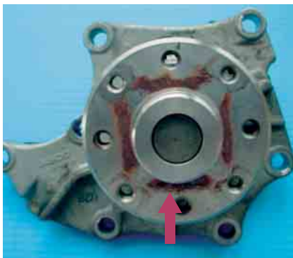
Flecking at the pulley seat
