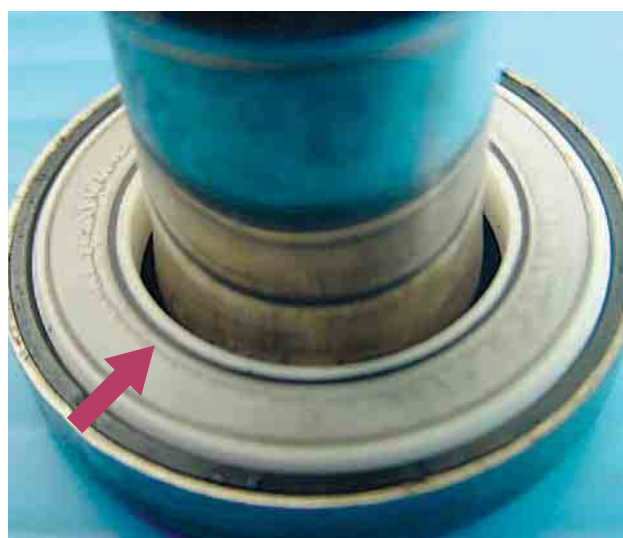
Damaged Accumulated sludge (Contaminated coolant).
