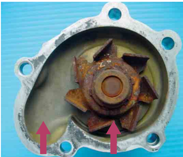
Contamination of water pump body Impeller corrosion
