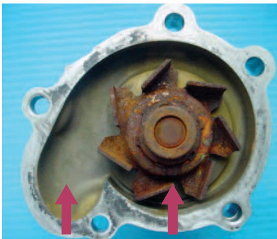
Contamination of water pump body
