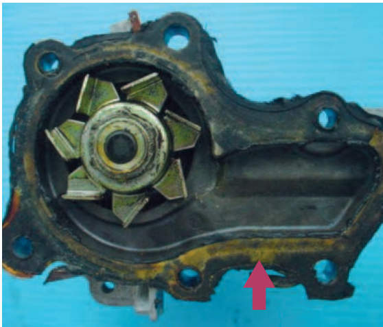
Insufficient accuracy on the mounting surface.
