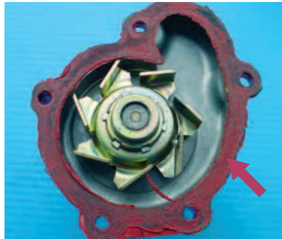
Gasket performance has degraded.
