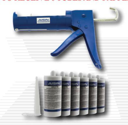
AB1217H is a high performance, room temperature vulcanized (RTV) sealant commonly used as a form-in-place gasket (FIPG). AB1217H has high elongation, low modulus, good elasticity, is oil resistant and blow-out resistant after curing. Good examples of usage for AB1217H are timing covers, valve covers, and oil pans.
